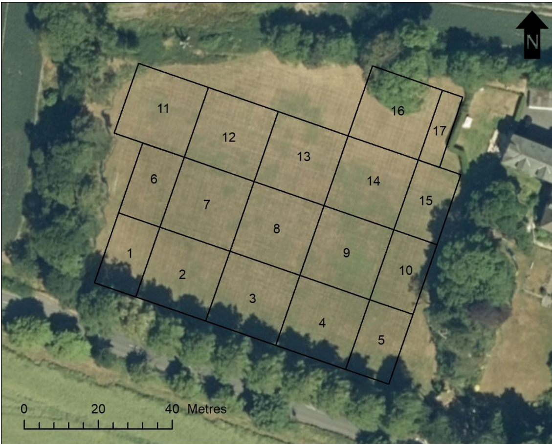
Figure 5 - Location and numbering of the gradiometer survey grids with 25cm AP as background
