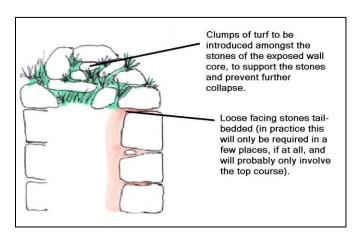
Fig. 1: schematic section across the curtain demonstrating clumped turfs supporting exposed stones of the core, stabilising the structure but maintaining a natural appearance.
