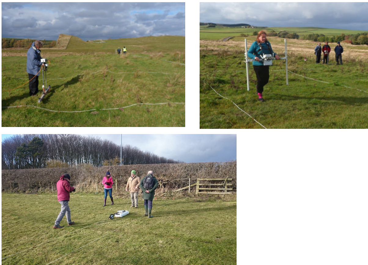
Fig 4.2. Geophysical survey methods. Top left: Soil resistance. Top right: Gradiometry. Bottom: Ground penetrating radar.
